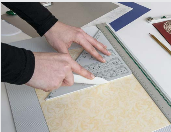
Making a scoring line along the line on one of the board's sides ensures nice fold of the paper.
